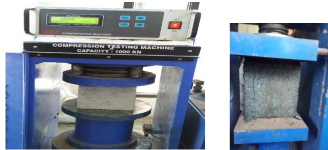
Figure.3 Setup for Compressive strength
