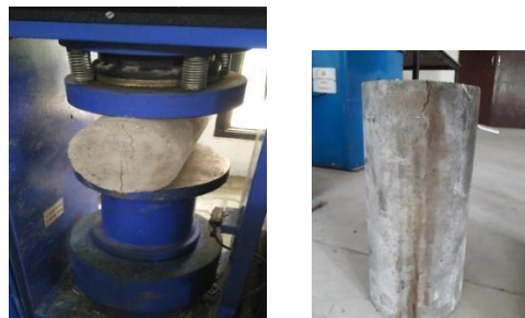
Figure.4 Setup for Split Tensile Strength
