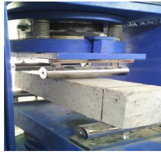
Figure.5 Flexure Strength Test
